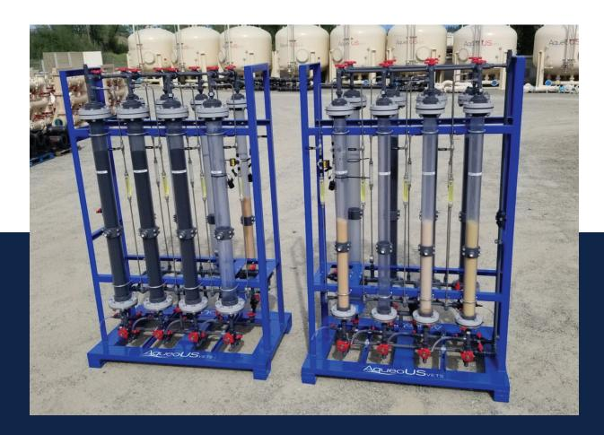
Testing filtration media just got easier. Ensure you are using the most efficient media based on your water quality with our on-site pilot equipment. Test up to eight different media types, replicating real-world fluid dynamics of empty bed contact time and hydraulic loading on a small scale.
