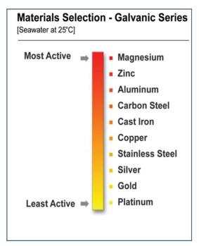
coating both cathodic and anodic metals to reduce the interaction between them<sup>1</sup>.
